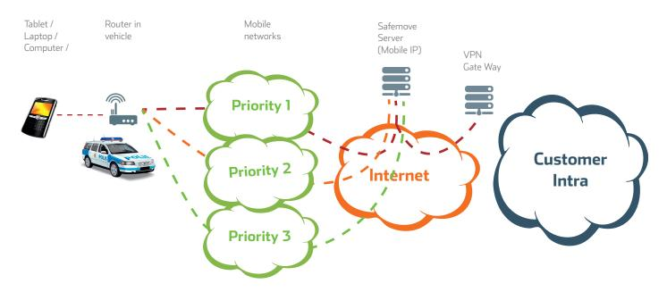
Each vehicle was equipped with a Multi-Channel Router (MCR) with selected available main operators in each case. A laptop or a tablet was attached to the router. The router created a Mobile IP tunnel to a server in the cloud and from there the connection to authorities' back-end systems was created. We wanted to test against the clarified customer claims. The first claim was that out in remote regions there is no network coverage at all. The second was that one operator is enough in the cities.
